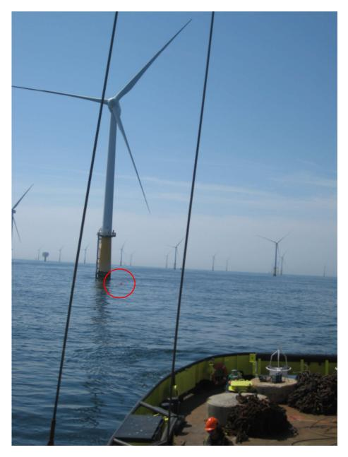
Figure 3.4 Deployment and recovery vessel 'Terschelling' near WTG1 Vestas V80 turbine. The orange and yellow floats, within the red circle, indicate position H1 with Sesame deployed.
