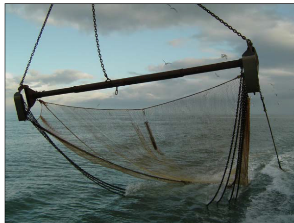
Figure 3-2: The 6m beam trawl, with the 20 mm DFS net. In the middle of the net, the CTD device is visible (Grift 2004).
