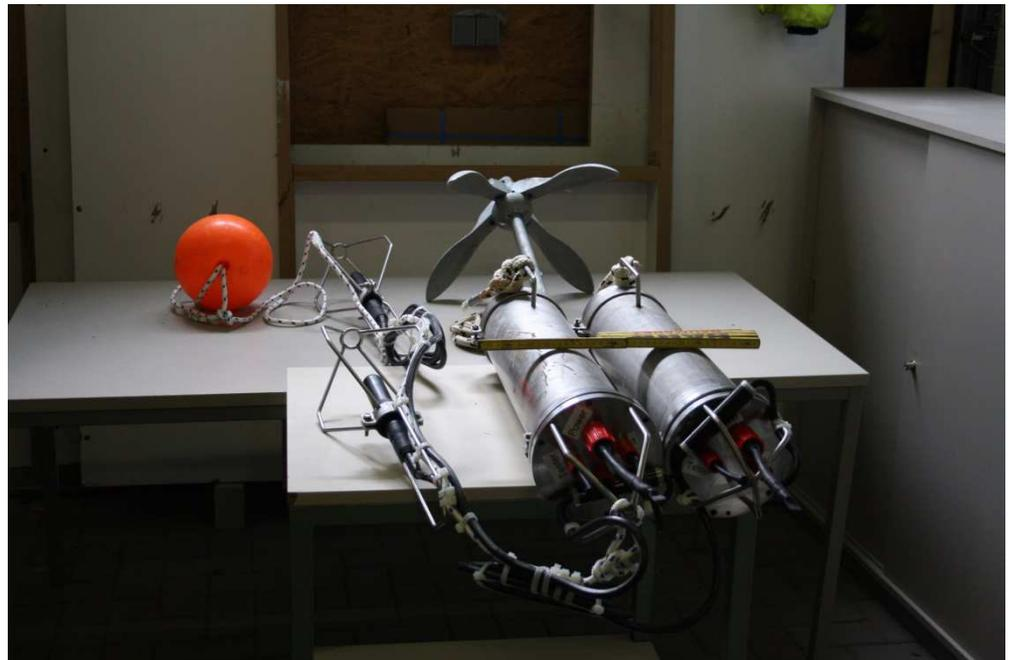
Figure B.1 Overview of ITAP system, two recorders with each its own hydrophone.
