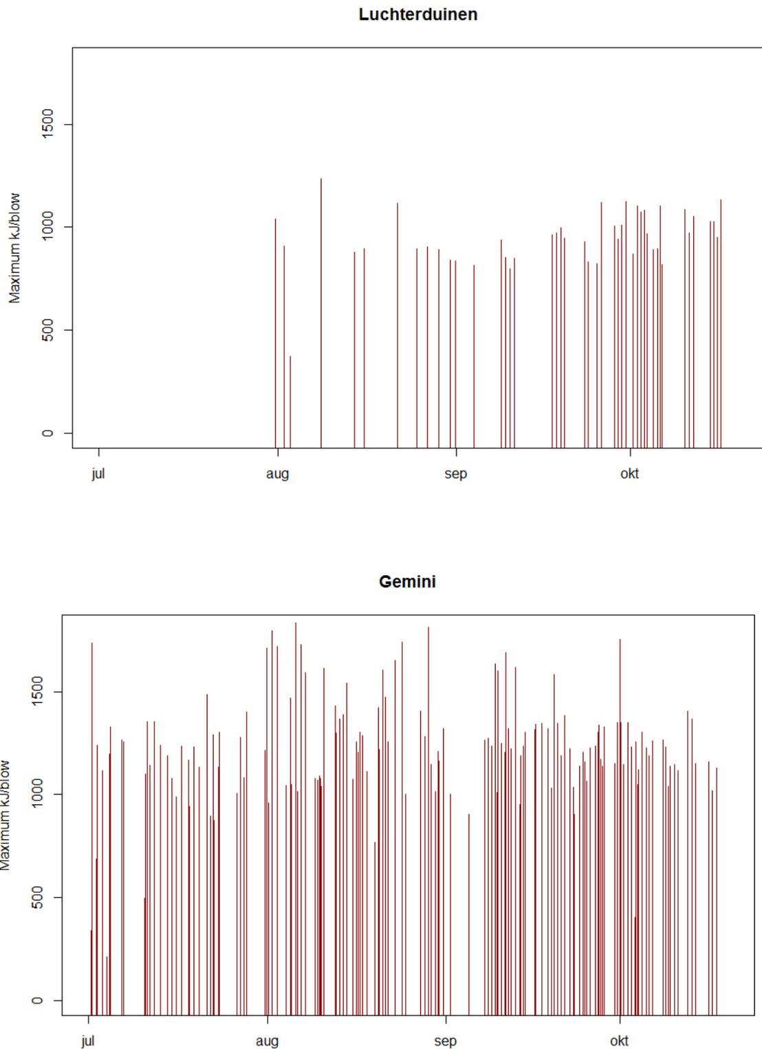
**Figure 1. Pile-driving activities (vertical red lines) for Luchterduinen in 2014 (upper figure) and Gemini in 2015 (lower figure).**
