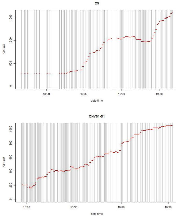
**Figure 2.** Examples of pile-driving logs from Luchterduinen (top two figures) and Gemini (bottom two figures). The red horizontal lines indicate energy level (kJ/blow). Vertical grey lines indicate start and stop times of a series of hammer blows with similar energy levels.
